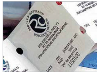
Cut and stack number added to pre-printed tickets in a narrow web flexo press application, printed by Domino A-Series
