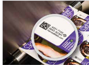
QR code printed on packaging by Domino K600i integrated on a rewinder
